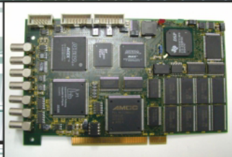
PSD data acquisition and accumulation block
