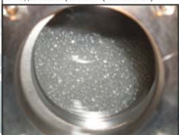
Beads of moderator material in the moderator chamber at 50 K (~27 000 pcs)
