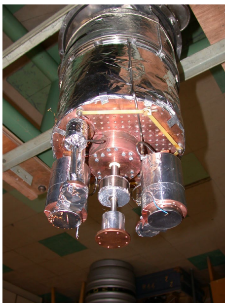
Fig. 3. The microrefrigerator with sorption pumping for temperatures down to 0.3 K.
