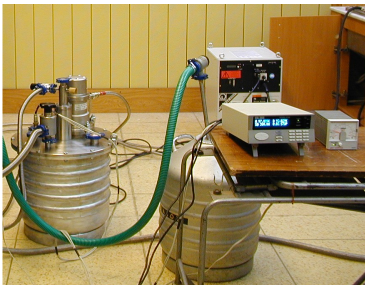
Fig 1. The close-cycle shaft cryostat on the basis of the two-step cryogenerator CoolPower 100T.
