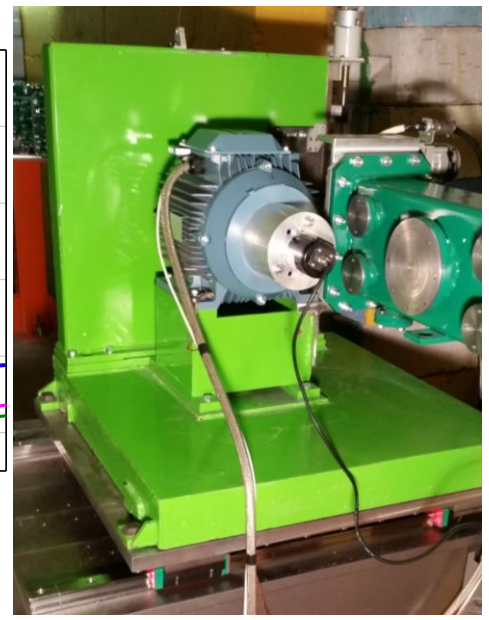
New F-chopper: \Omega_{\max}=6000 \text{ rpm}
