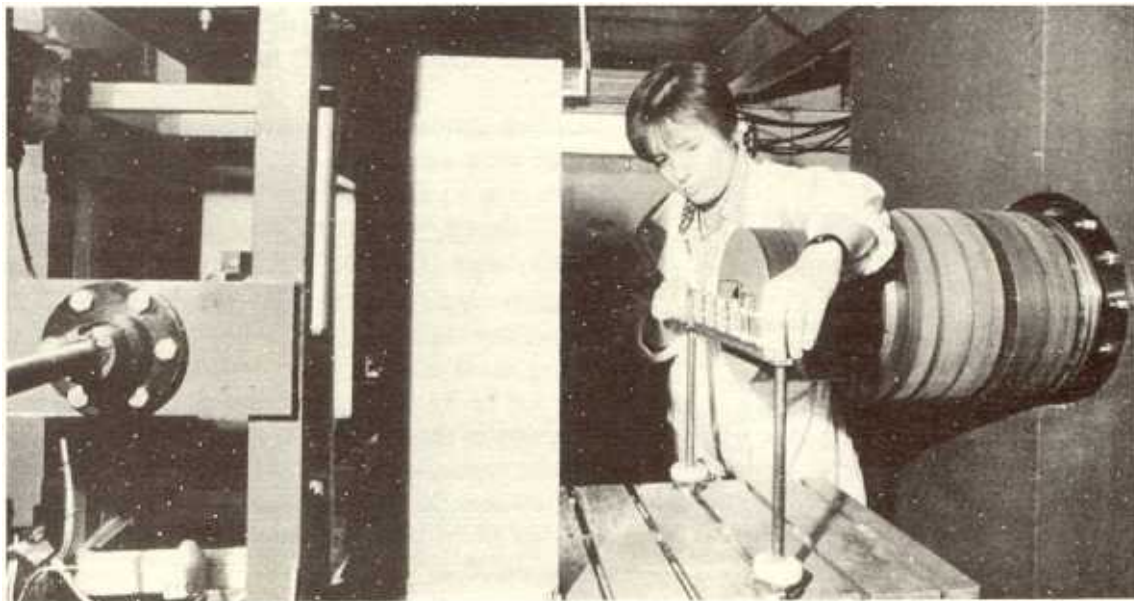
MURN small-scattering diffractometer on beam 4 at the IBR-2 reactor
