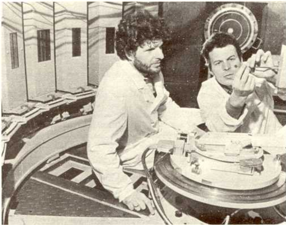
HRNS texture neutron diffractometer on beam 7a at the IBR-2 reactor
