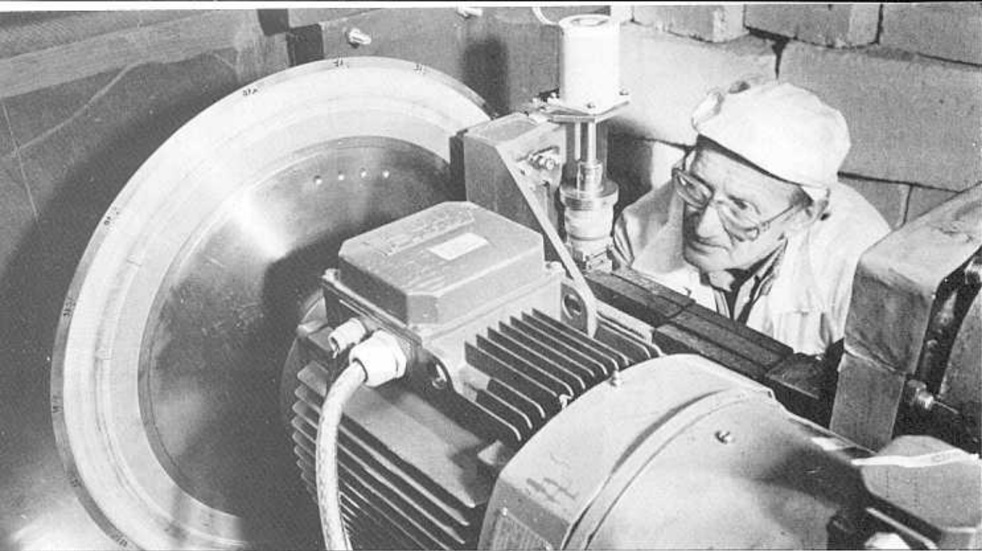
V.G.Simkin tunes the control system of the Fourier chopper.
