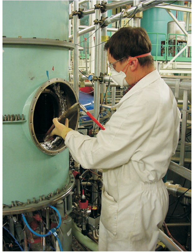
A.V.Strelkov installs samples for measuring UCN small heating (ILL, Grenoble, France).
