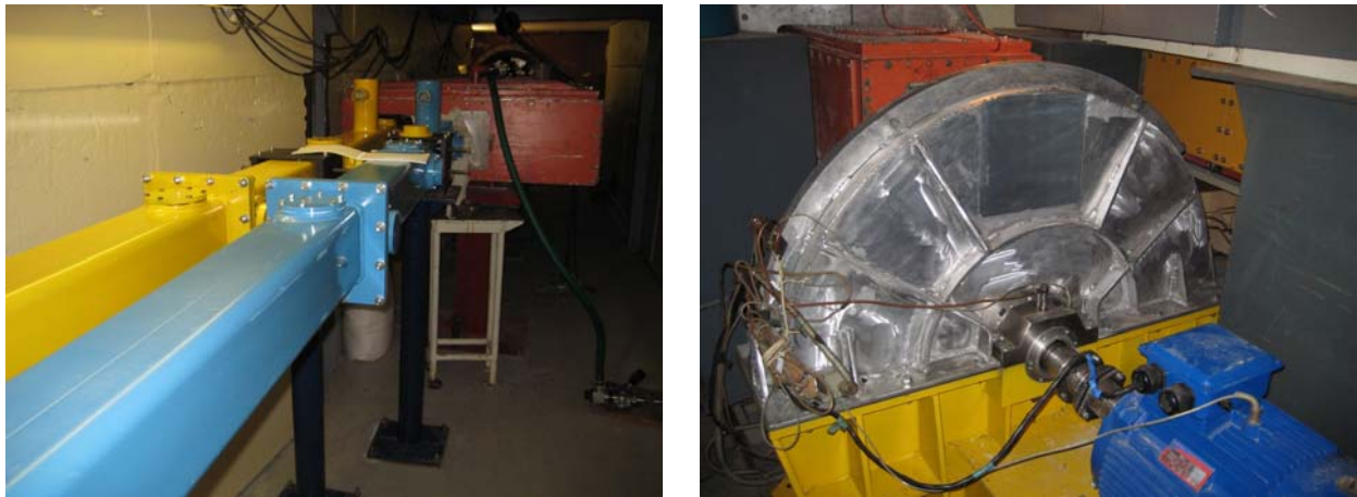
Fig. 14. The splitter dividing the initial neutron beam into three independent beams for the EPSILON, SKAT and NERA spectrometers (left) and the new background chopper (right) on beam 7 of the IBR-2 reactor.
