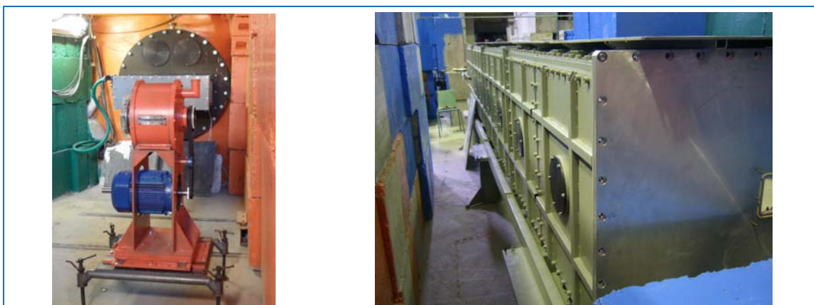
Fig. 13. Left: background neutron chopper for the GRAINS reflectometer at its regular place in the IBR-2 experimental hall. Right: beam-forming system of the GRAINS reflectometer in the IBR-2 experimental hall.
