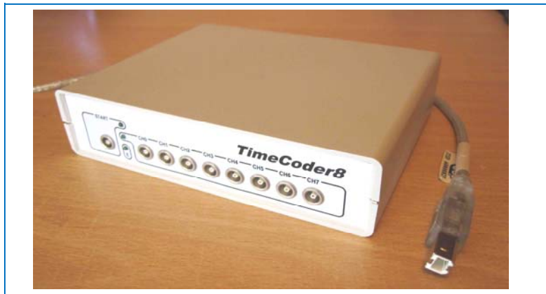
Fig. 21. An overall view of 8-channel time encoder.
