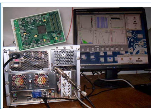
Fig. 18. ADC ADCM16-LTC 16-channel system.
