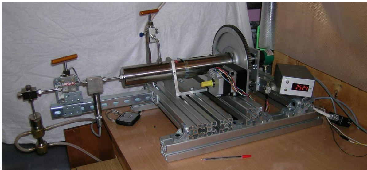
Fig. 1. Volumetric high-pressure setup of the YuMO spectrometer, adapted for SANS experiments.
