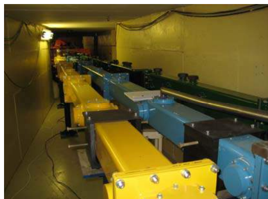
Fig. 1 (left): Set-up of the neutron guide system at beamline 7 of the pulsed source IBR-2M.
