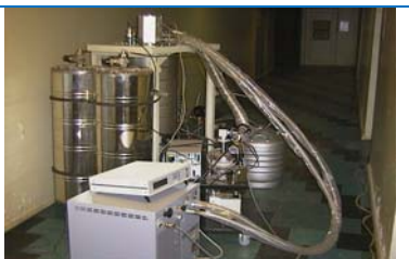
Fig. 31. Helium-3 purification facility.
