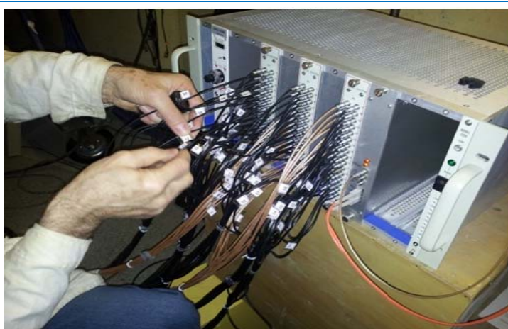
Fig. 37. Photo of MPD-32 electronic modules.
