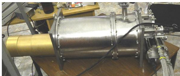
Fig. 50. Horizontal cryostat for the DN-6 diffractometer.
