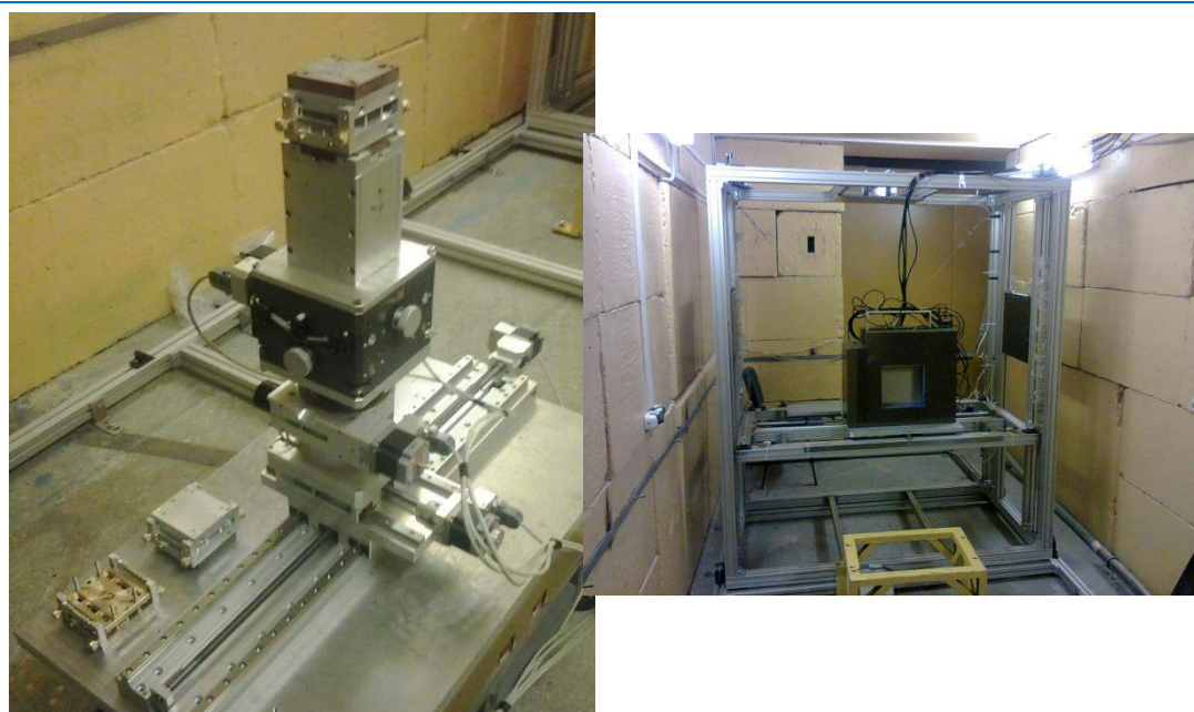
Fig. 17. Sample table with a liquid cell (left) and automatic movable platform for the detector (right).
