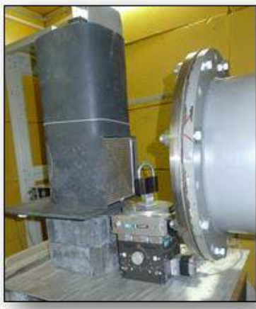
Fig. 18. Spectrometer for neutron radiography and tomography on IBR-2 beamline 14.
