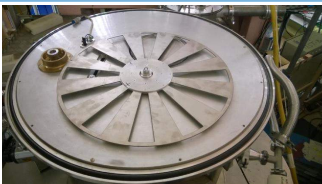
Fig. 53. Multi-slit Fourier-chopper of the Epigraph spectrometer.
