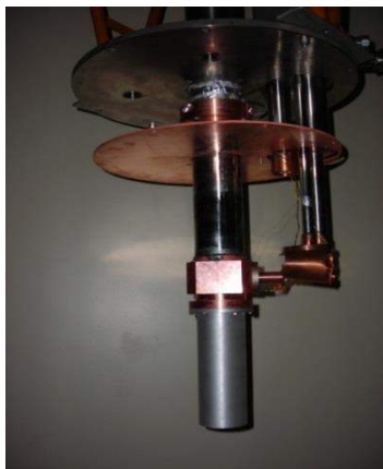
Fig. 71. Shaft cryostat for the NERA-PR spectrometer.
