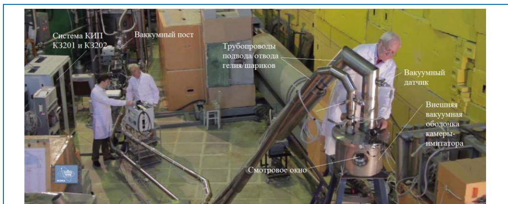
Fig. 56. Full-scale stand of CM-201 (control and measurement equipment of CM-201 and CM-202; vacuum station; helium/bead feed/discharge pipes; observation window; vacuum sensor; outer vacuum jacket of simulator chamber).
