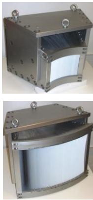
Fig. 1-I-25. New wide-aperture radial collimators for the FSD Fourier diffractometer, beamline 11A of the IBR-2 reactor (a). Bulk sample under study on the HUBER goniometer at FSD. Small scattering volume (gauge volume) within a sample is cut by the radial collimators mounted on special adjusting frames (b).
