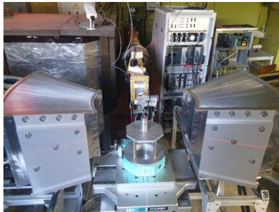
Fig. 1-I-25. New wide-aperture radial collimators for the FSD Fourier diffractometer, beamline 11A of the IBR-2 reactor (a). Bulk sample under study on the HUBER goniometer at FSD. Small scattering volume (gauge volume) within a sample is cut by the radial collimators mounted on special adjusting frames (b).
