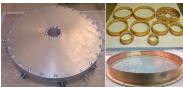
Fig. 1-IV-12. Photos of the housing (left), internal part of the detector and 9 independent coaxial rings (right).
