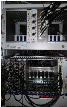
Fig. 1-IV-17. Electronics of high-voltage power supply of detectors (top crate), modules of detector electronics and data acquisition electronics (bottom crate).
