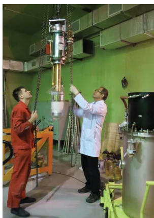
Fig. 1. Assembling of modulators and klystrons; the modulator during tests.
