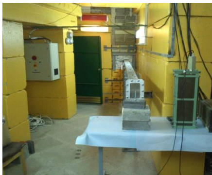
Fig. 9. The exit section of the neutron guide on IBR-2 beamline 13.
