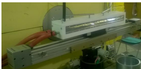
Fig. 21. Device for horizontal positioning of samples at the YuMO spectrometer (left).
