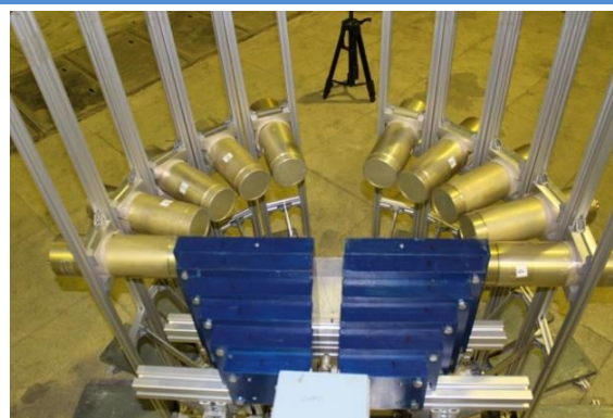
Fig. I-3-13. System with 10 detectors, configuration variant "A" – compact geometry with a collimator.
