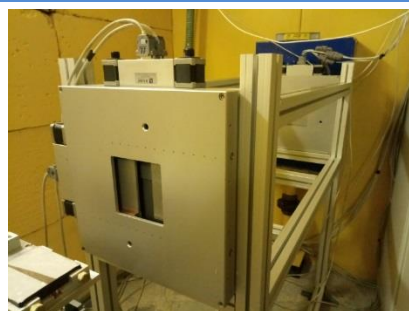
Fig. II-1-5. Controllable slit-type apertures for collimating beam directly at the sample position on the GRAINS reflectometer.
