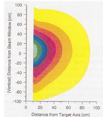
**Fig. 4.3:** Contours of the unperturbed thermal neutron flux in the SINQ-moderator tank at 1 mA proton current, for a massive lead target with low absorption container: the highest flux is in the centre near the beam window with  $1.9 \times 10^{14} \text{ n/cm}^2 \text{ s}$  (light green), decreasing in steps of  $0.2 \times 10^{14} \text{ n/cm}^2 \text{ s}$  for each consecutive coloured zone to  $1 \times 10^{13} \text{ n/cm}^2 \text{ s}$  (yellow) at the edge.
